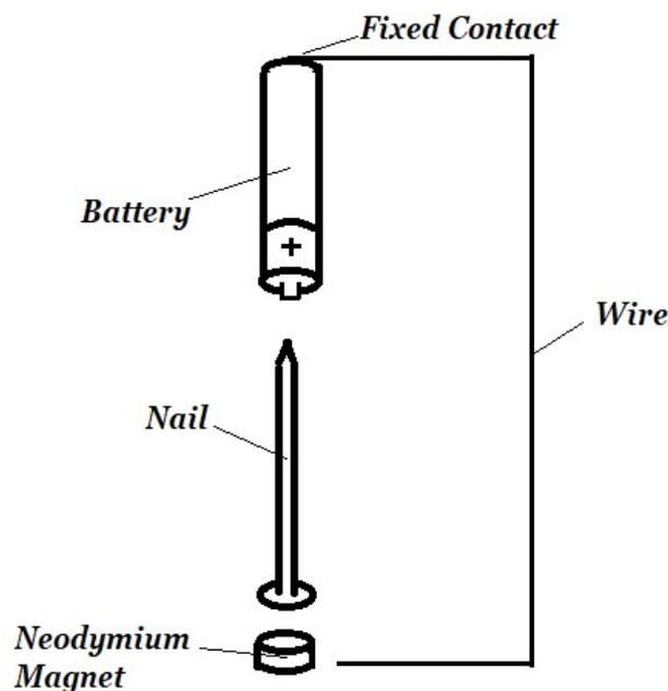
When the wire makes contact with the neodymium magnet the nail and magnet will spin. The longer they're in contact, the faster they will spin.
